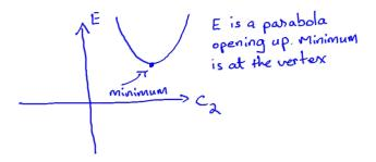
The minimum is at the vertex, and the vertex of  $E = ac_2^2 + bc_2 + c$  occurs at  $c_2 = -b/(2a)$  (result from section 2.1), so we have
