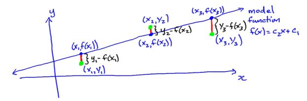
We choose to make the *best fit line* to be the one that makes the sum of all the vertical distances as small as possible (minimize):
