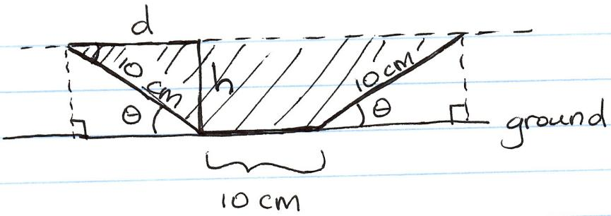
Cross section of gutter determines how much water gutter can hold.
